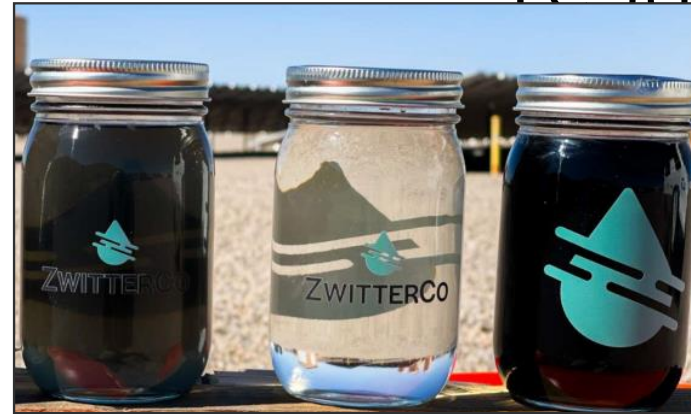
Permian Basin -100,000 TDS PW (left) w/membrane pre-treatment and concentrate (right)
