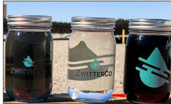
Permian Basin -100,000 TDS Raw PW (left) pre-treatment (center)
